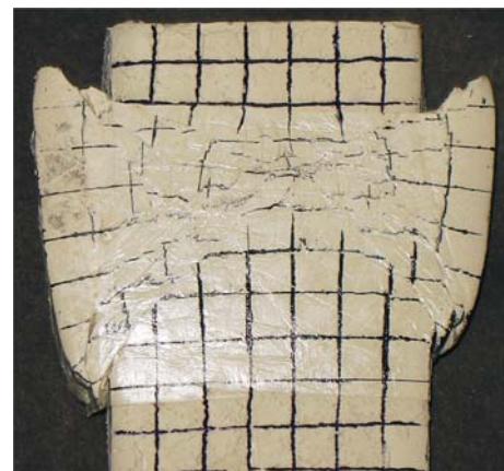
Figure 5. Deformed clay sample at the end of the test (at 16% axial strain).
