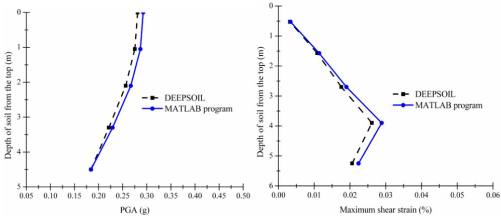
Fig. 5 Peak acceleration and maximum shear strain with depth for Trombay site in equivalent linear domain.
