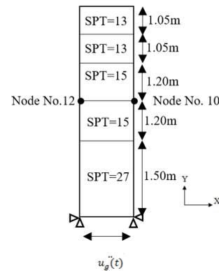
Fig. 3 Schematic diagram of soil column for Trombay in Mumbai city.
