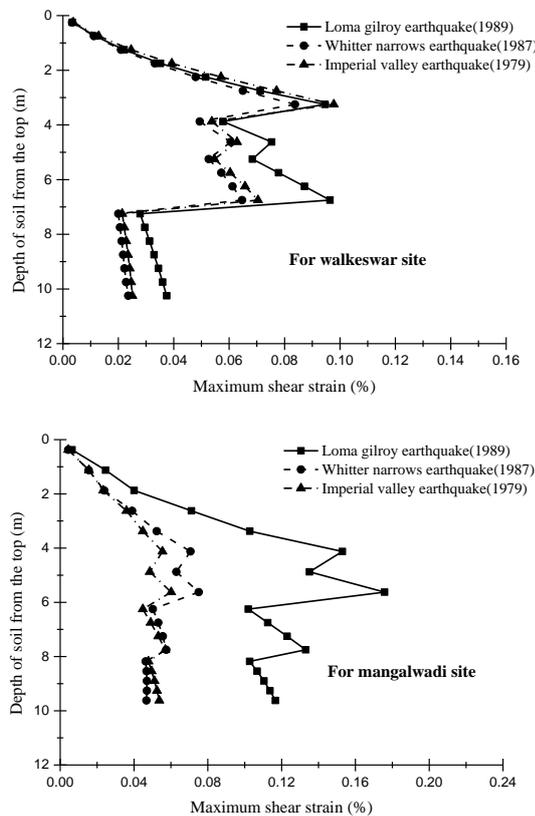
Fig. 11 Variation of maximum shear strain in soil with depth at Walkeswar and Mangalwadi sites
