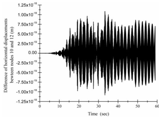
Fig. 6 Difference between the horizontal displacements at Nodes 10 and 12
