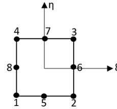
Fig. 1 Node numbering in a 8-noded quadratic quadrilateral element.
