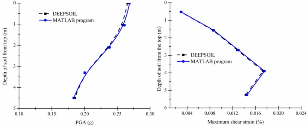
Fig. 4 Peak acceleration and maximum shear strain with depth for Trombay site in elastic domain.
