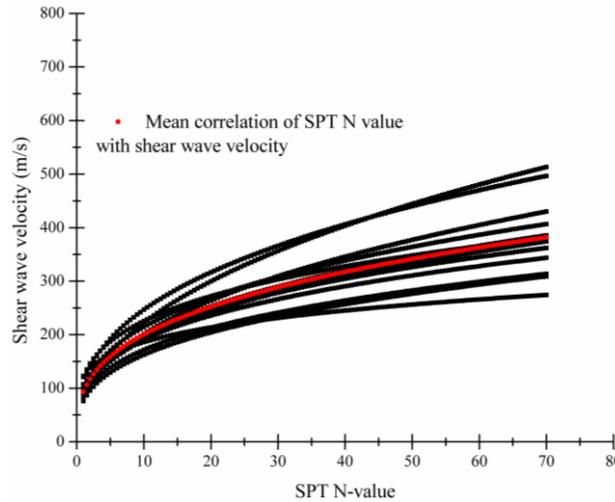
Fig. 2 Variation of shear wave velocity of soil with N-value for Mumbai city
