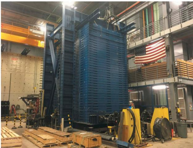
**Figure 4.** Geotechnical laminar box test setup.
