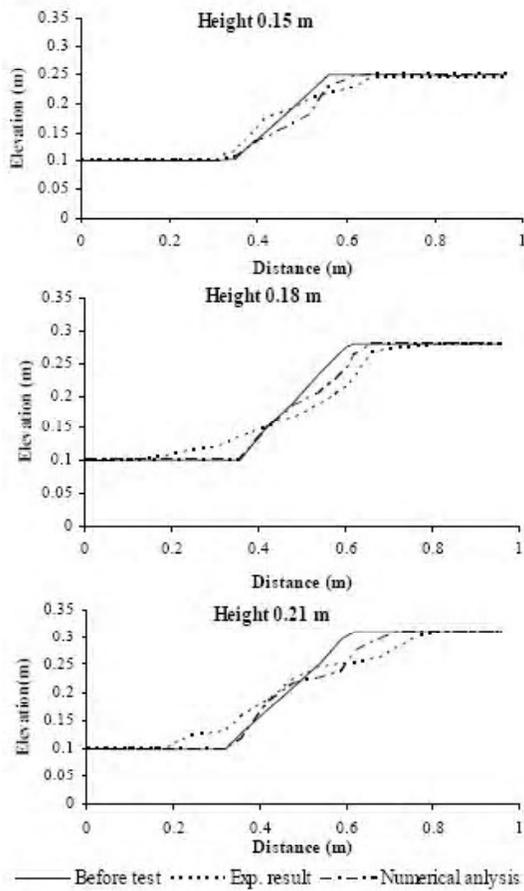
Fig. 5: Side Profile of Failed Model Slopes
