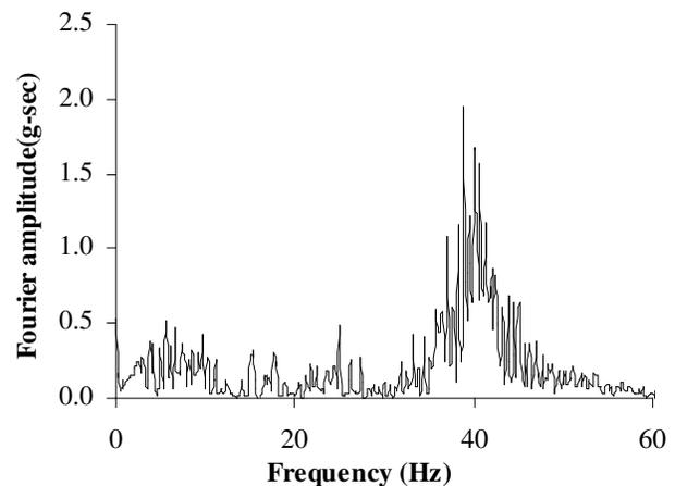
**Fig. 4:** Frequency Content of the Whole Test Setup with Soil Slope
