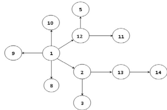
Figure 14. Machining precedence constraints for the example part
