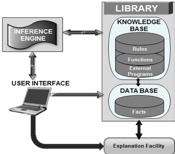
Figure 2. Architecture of the CLIPS Expert System Shell
