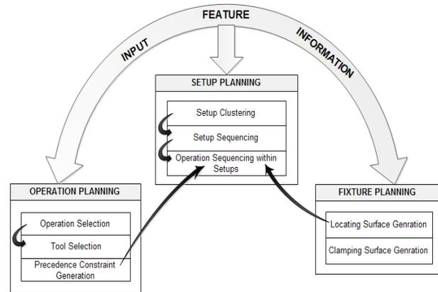
**Figure 1.** Data interactions between the components of the Process Planning System
