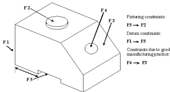
**Figure 6.** Illustration of different machining precedence constraints
