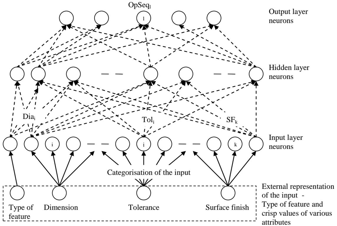
**Figure 2. Topology of the proposed neural network model**
