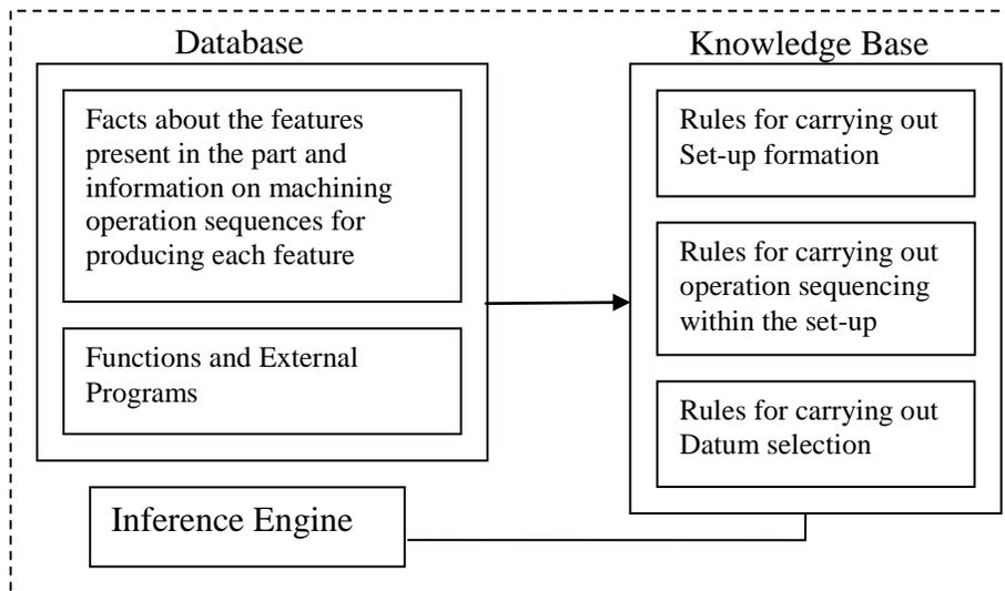
**Figure 3. Overall structure of the set-up planning module which is based on expert system**
