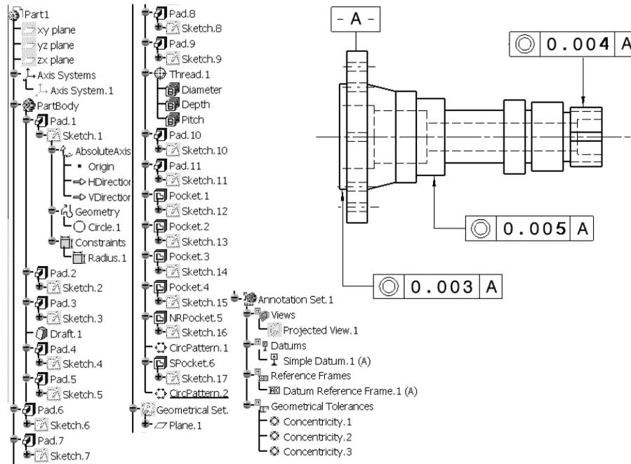
Figure 11. Feature Tree of the Part in CATIA with details of Pad.1
