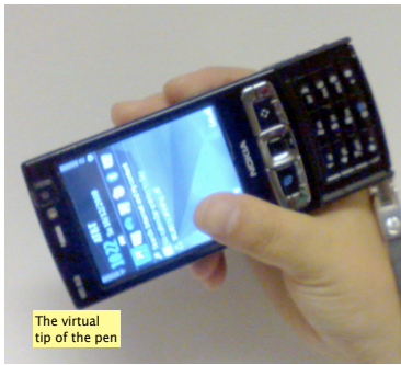
Figure 2: (a) Pretending the phone’s corner to be the pen-tip reduces rotation. (b) Raw accelerometer data while drawing a rectangle (note gravity on the Z axis). (c) Moving average computation.
