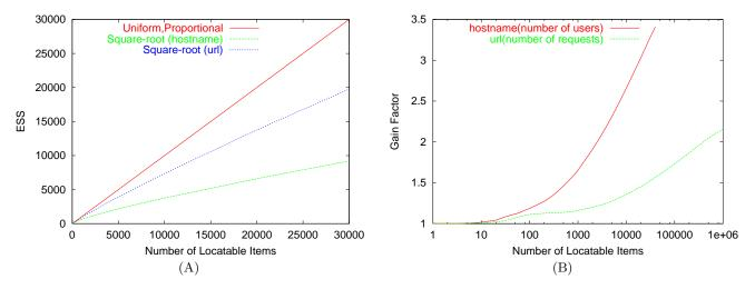
Figure 3: (A) The ESS of the different strategies versus the number of locatable items m (the x axis), for the hostname and Url distributions. (B) The gain factor as a function of m for the two distributions.
