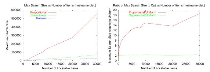
Figure 4: Maximum search size as a function of number of locatable items, and ratio of maximum search size to the minimum possible (Uniform allocation).
