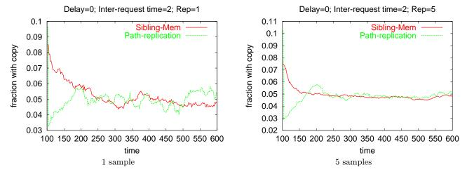
Figure 6: Simulating performance of Path Replication and Sibling-Memory algorithms. In these simulations there is no delay in copy creation; the copy lifetime is 100 time units; and the inter-request-time is 2 time units
