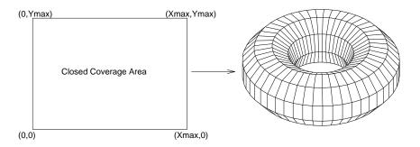
Figure 7: Rectangular simulation area mapped to a torus in the Boundless Simulation Area Mobility Model.
