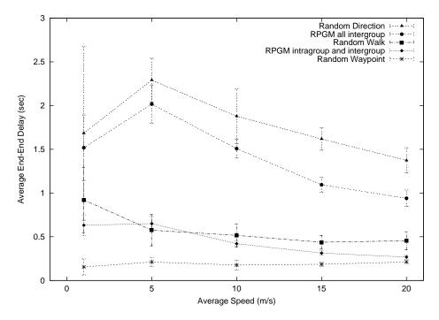
Figure 22: End-to-end delay vs. speed.
