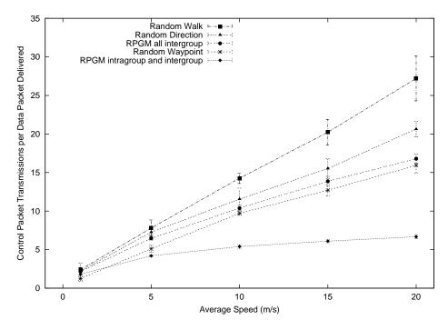
Figure 24: Control packet overhead vs. speed.
