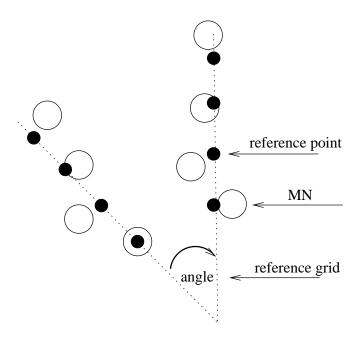
Figure 14: Movements of three MNs using the Column Mobility Model.
