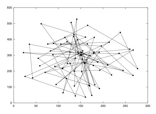
Figure 1: Traveling pattern of an MN using the 2-D Random Walk Mobility Model (time).
