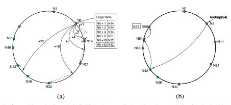
$Fig.\ 4.\ (a)\ The\ finger\ table\ entries\ for\ node\ 8.\ (b)\ The\ path\ a\ query\ for\ key\ 54\ starting\ at\ node\ 8,\ using\ the\ algorithm\ in\ Figure\ 5.$
