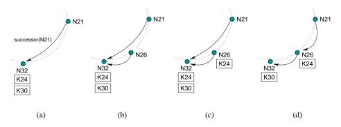
Fig. 7. Example illustrating the join operation. Node 26 joins the system between nodes 21 and 32. The arcs represent the successor relationship. (a) Initial state: node 21 points to node 32; (b) node 26 finds its successor (i.e., node 32) and points to it; (c) node 26 copies all keys less than 26 from node 32; (d) the stabilize procedure updates the successor of node 21 to node 26.
