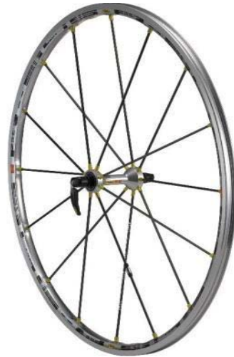
Fig: spokes of a bicycle wheel in pretension
