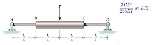
4. The bar is supported by a roller constraint at B which allows vertical displacement but resists axial load and moment. If the bar is subjected to the loading shown, determine the slope at A, and the deflections at B and C.  $\left[-\frac{3PL^2}{8EI}, -\frac{11PL^3}{48EI}, -\frac{PL^3}{6EI}\right]$
