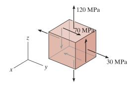
13. For the state of stress, determine the maximum shearing stress when (a)  $\sigma_z = 0$ , (b)  $\sigma_z = 60$  MPa, (c)  $\sigma_z = -60$  MPa. [(a) 113.0 MPa, (b) 91.0 MPa, (c) 143.0 MPa]
