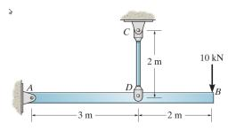
7. Determine the displacement at point C and the slopes at C and A.  $\left[\frac{2Pa^3}{3EI}, \frac{5Pa^2}{6EI}, \frac{Pa^2}{6EI}\right]$
