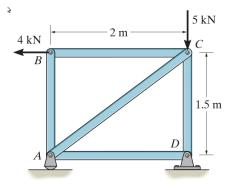
4. Determine the horizontal displacement of joint B of the truss. Each steel member has E = 200 GPa and A = 1935 mm<sup>2</sup>. [0.753 mm]
