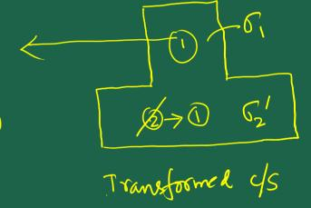
10. The reinforced concrete beam shown is subjected to a positive bending moment of 175 kN·m. Knowing that the modulus of elasticity if 25 GPa for the concrete and 200 GPa for the steel, determine the stress in the steel and the maximum stress in the concrete.
