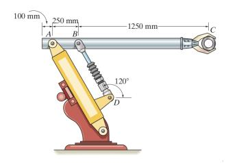
3. Draw the shear and moment diagrams for the overhanging beam.
