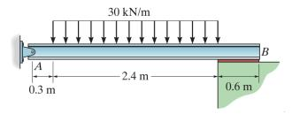
5. Draw the shear and moment diagrams for the beam when the support at A allows it to slide freely along the vertical guide and hence it cannot support a vertical force.
