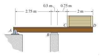
8. The compound beam is fixed at A, pin connected at B, and supported by a roller at C. Draw the shear and moment diagrams for the beam.
