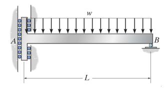
6. The shaft is supported by a smooth thrust bearing at A and a smooth journal bearing at B. Draw the shear and moment diagrams for the shaft.
