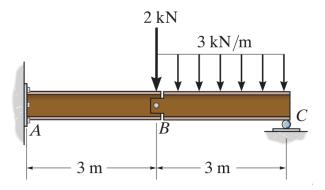
10. Draw the shear and bending moment diagrams for the beam and loading shown.
