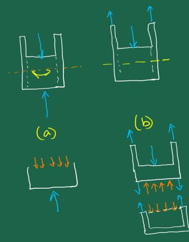
5. The thin-walled cylindrical pressure vessel shown in the figure is subjected to an internal gauge pressure of 15 MPa. If the thickness is 10 mm, and the material constants are E=200 GPa and  $\nu=0.3$ , determine the increase in both the diameter and the length of the pressure vessel. [3.19 mm, 2.25 mm]
