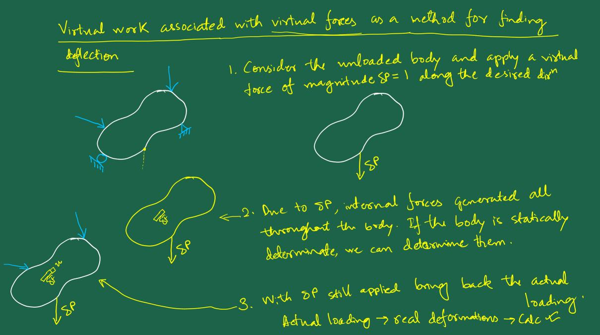
4. Write the end. virtual work by multiplying SP with Dire the deformation along the desired dir.
