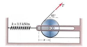
5. The spring of modulus k=3.5 kN/m is stretched 10 mm when the disk center O is in the leftmost position x=0. Determine the tension T required to position the disk center at x=150 mm. At that position, what is the normal force N exerted on the horizontal frictionless guide? The mass of the disk is 3 kg.
