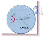
3. The 100 kg wheel rests on a rough surface and bears against the frictionless roller A when the couple M is applied. If M=60 Nm and the wheel does not slip, compute the reaction on the roller A.
