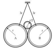
8. Two identical smooth tubes A and B, each of weight W, are suspended at their ends by cords of equal length. A third tube C of weight  $W_c = 0.8W$  is placed between A and B. Determine the greatest weight of C that can be supported without upsetting equilibrium.
