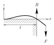
Assume that the weight of the beam itself is negligible compared with F. Based on the principle of virtual work show that the beam deflection w(x) will be governed by the following governing differential equation:
