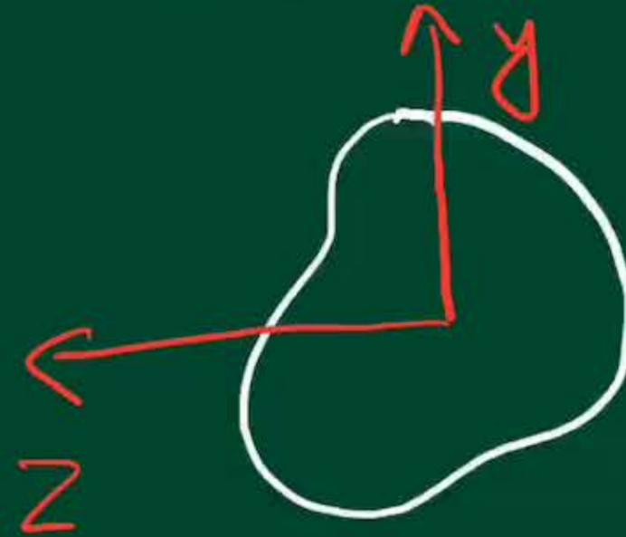
If the axes are so chosen that  $I_{yz} = 0$  then the axes are referred to as principal axes.
