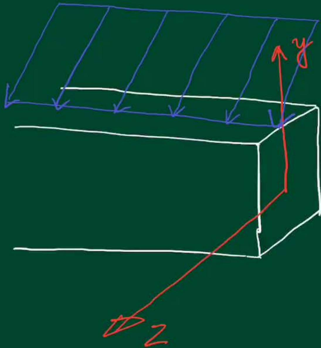
2nd CASE OF UNSYMMETRIC BENDING: C/S IS UNSYMMETRIC
