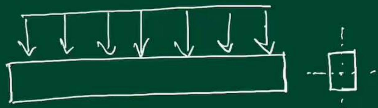
SYMMETRIC BENDING OF BEAMS
