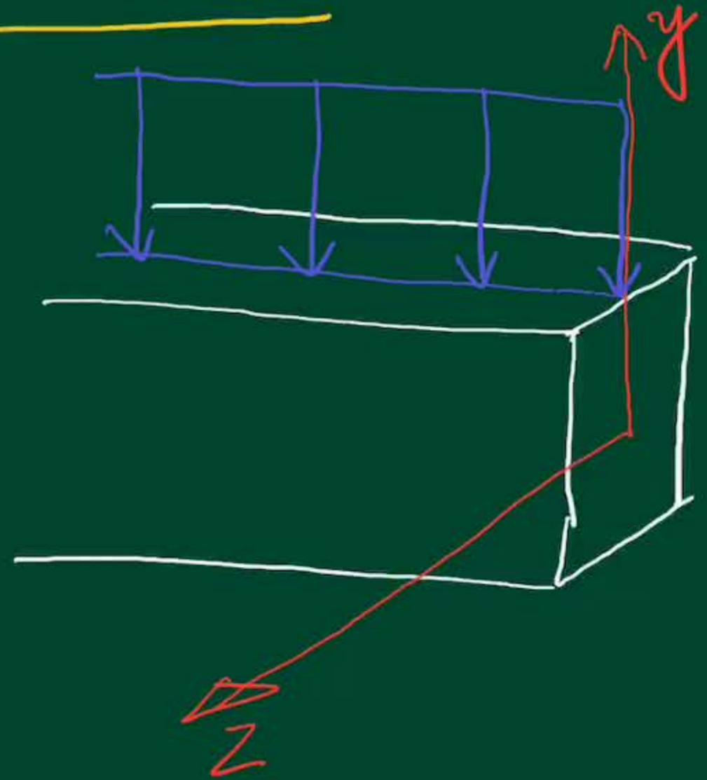
1st CASE OF UNSYMMETRIC BENDING: C/S IS SYMMETRIC BUT LOADING IS UNSYMMETRIC
