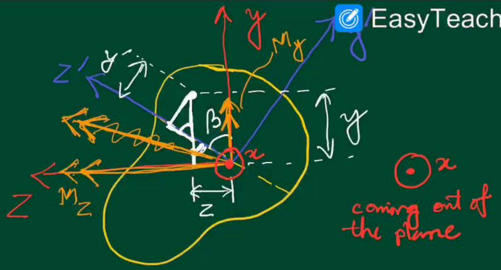
We understand that under pure bending the bending stresses denoted by  $\sigma_{xx}$  will have a linear distribution about the  $z'$  axis (i.e. about the N/A)
