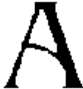
Erosion by 3*3 square structuring element
