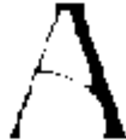
Erosion by 5*5 square structuring element
