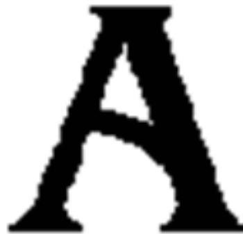
Dilation by 3 \times 3 square structuring element
