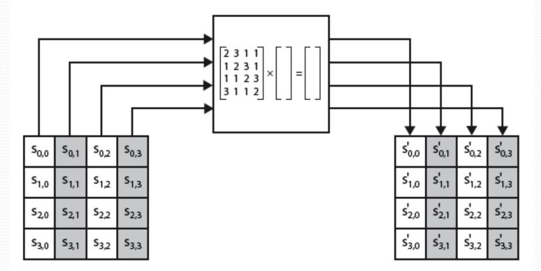
The MixColumns transformation operates at the column level; it transforms each column of the state to a new column.
