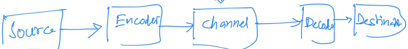
Block diagram of a communication system.
