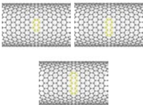
Figure 6 Zigzag SWNTs with 1,2 and 3 bonds cut
