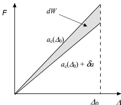
Figure 3 Displacement-controlled fracture test
