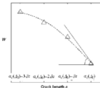
Figure 5 External work-Crack length ( $W$ - $a$ ) curve for SWNTs
