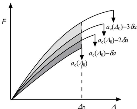
Figure 4 Method used in this study for determining strain energy release rate
