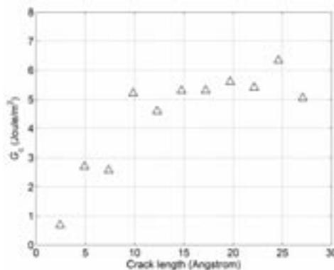
Figure 8 Critical strain energy release rate for (35,0) SWNT at 300 Kelvin
