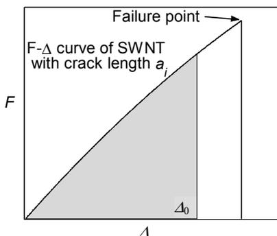
Figure 2 Force-Displacement curve of a tensile test of a SWNT with crack length  $a_i$ . The shadowed area is  $W$ , the work done by the external force
