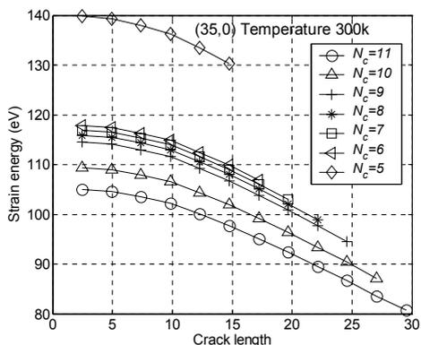
Figure 7 External work-crack length ( $W-a$ ) curve for (35, 0) SWNT at 300 K
