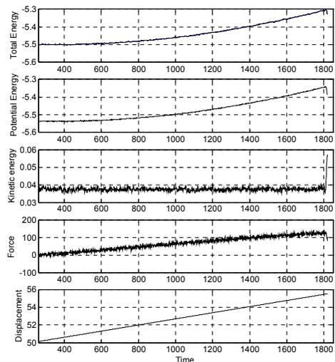
Figure 1. Time histories of total energy, potential energy, kinetic energy, force and displacement from atomistic simulation of a (35,0) SWNT to fracture
