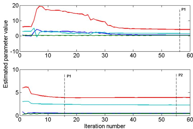
**Figure 2: Comparison based on rate of convergence criteria for parameter identification between conventional filtering methods using constant covariance matrix (top) and using the adaptive scheme for covariance (bottom). P1 and P2 are the preset precision points. Four lines are due to four parameters  $\alpha$  (Blue),  $\beta$  (Red),  $\gamma$  (Green) and  $n$  (cyan).**
