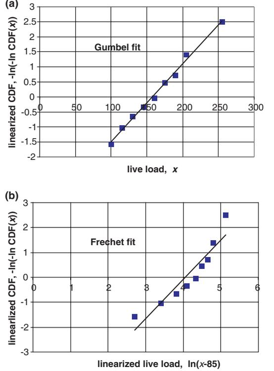
Figure 3. (a) Gumbel and (b) Frechet probability fit of daily maximum of the associated i.i.d. live-load sequence.
