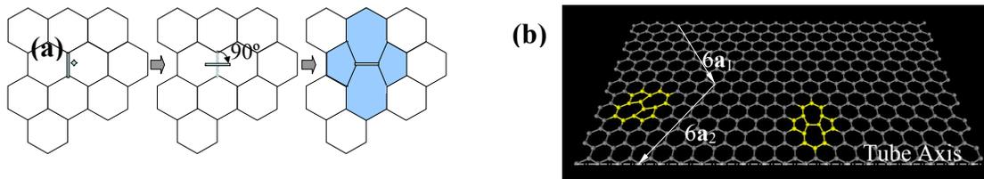
**Figure 1 (a) Rotation of carbon bonds to form SW defects (b) graphene sheet with 2 random defects ( $a_1$  and  $a_2$  are unit vectors and  $(m,n)$  is the tube charity)**
