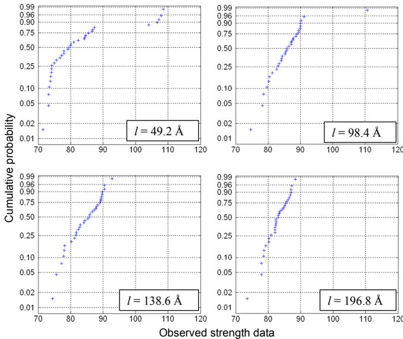
**Figure 3 Goodness of Weibull fit for SWNT ultimate strength with increasing tube length (33 samples each)**
