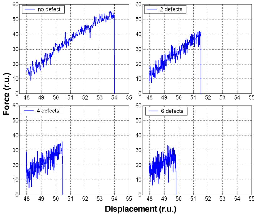
**Figure 2 Force-displacement curves of nanotubes with various number of defects**
