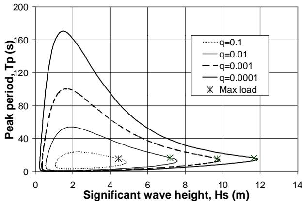
**Figure 3: Hs-Tp contours and locations of maximum connector axial load**
