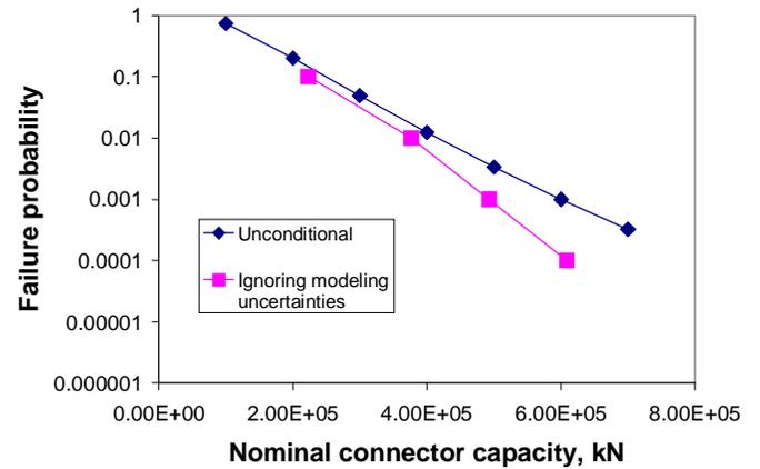
**Figure 4: Connector failure probability**
