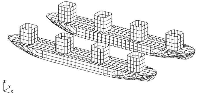
Figure 2: Hydrodynamic panel model of one MOB module
