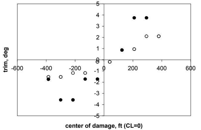
Figure 1 Sinkage as a function of the damage parameters (○ = one-compartment flooding, ● = two-compartment flooding)
