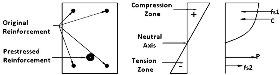
Fig. 1. Force balance and moment computations for partially prestressed section.
