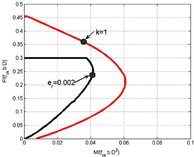
**Fig. 4.** P–M interaction diagram between inplane compressive force and moment capacity – black (inner) = cracking, red (outer) = collapse. (For interpretation of the references to color in this figure legend, the reader is referred to the web version of the article.)
