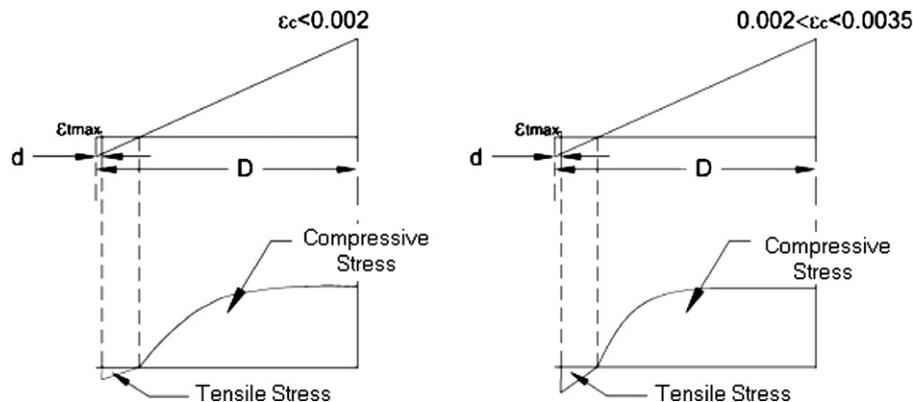
Fig. 3. Strain and stress distributions on section for  $\epsilon_c < 0.002$  (left) and  $\epsilon_c > 0.002$  (right) for limit state of cracking.
