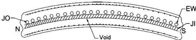
**Fig. 5.** Prestressed concrete shell.
