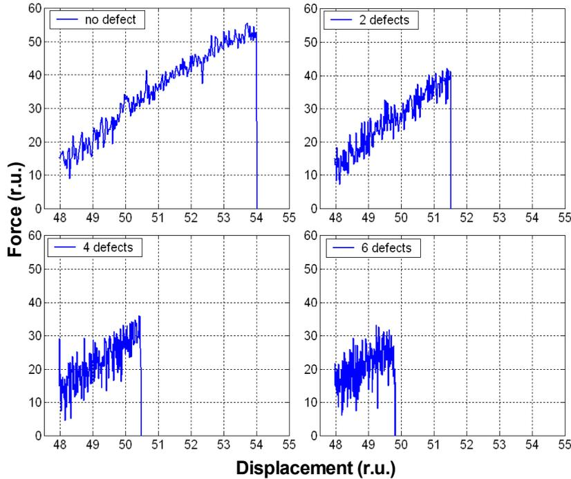
**Figure 4 Force-displacement curves of nanotubes with various defect intensities**
