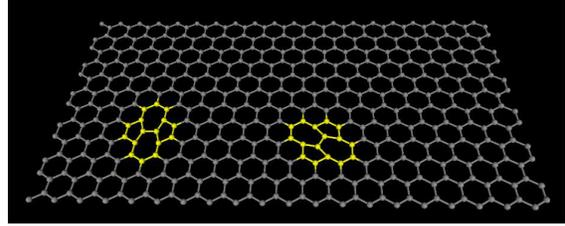
**Figure 3** Graphene sheet with 2 random distributed defects
