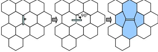
**Figure 2** Rotation of carbon bonds to form SW defects
