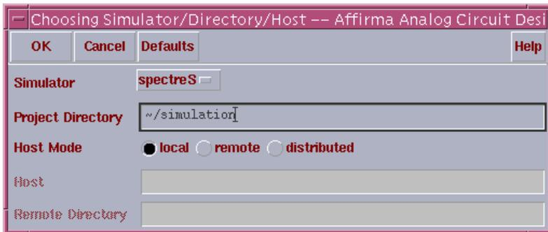
Note: If the simulator cdsSpice is chosen, the setup procedure is the same as SpectreS. If the simulator Spectre is chosen, the setup is different from SpectreS and the details will be shown in Appendix.
