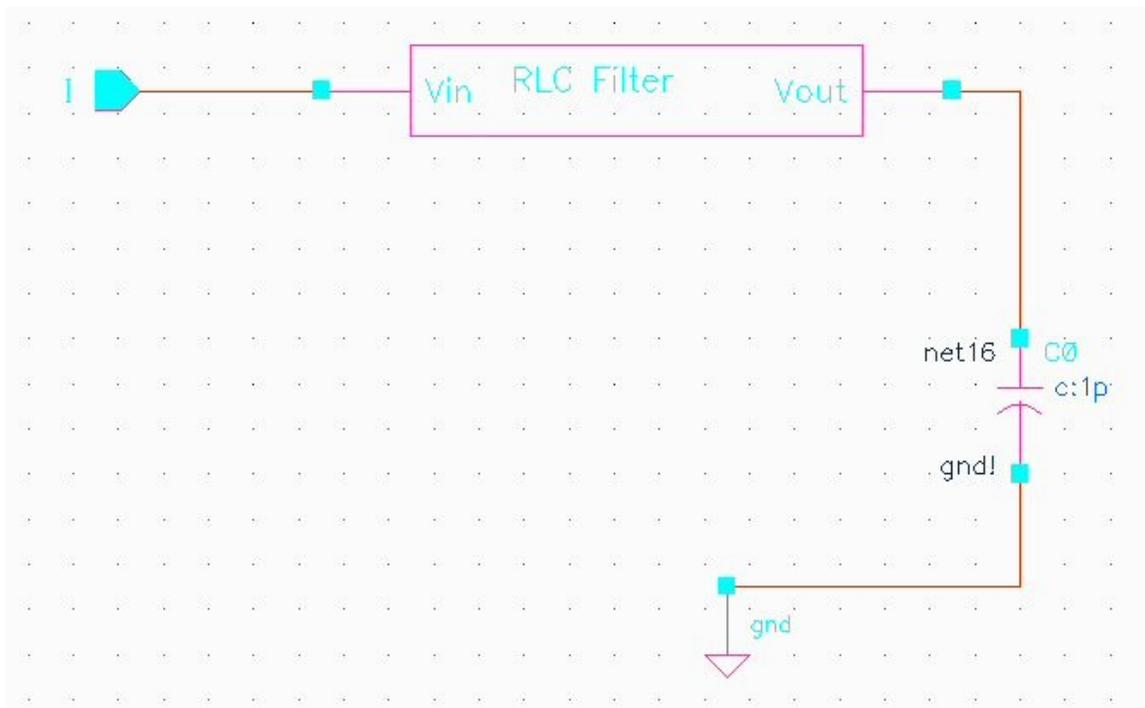
Test Circuit for Simulation with Spectre
