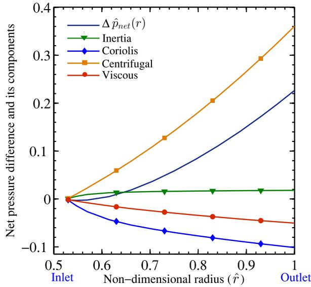
FIG. 8. Radial variation of local net pressure difference  $\Delta\hat{p}_{net}(r)$  and its components: prediction of the present CFD simulations for radial outflow. ( $\hat{r}_i = 0.528, \hat{b} = 0.008, Ds = 1, \phi = 0.124$ , and uniform velocity distribution at inlet:  $U_{r,i} = \bar{U}_{r,i}$ . Pressure differences are non-dimensionalized by  $\rho\Omega^2 r_o^2$ . There are 125 grid points between the inlet and the outlet.)
