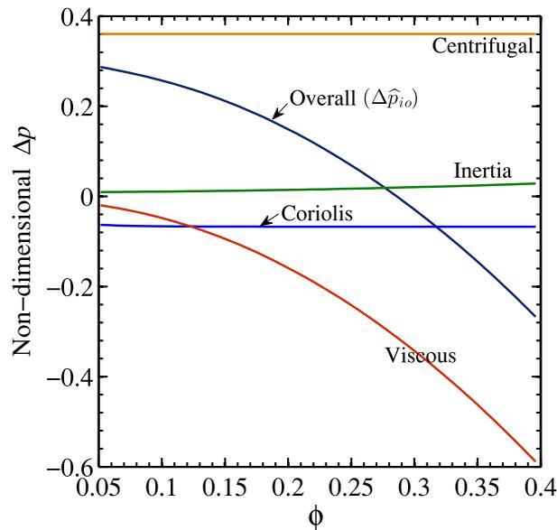
FIG. 7. Contribution of various forces to produce the overall radial pressure difference  $\Delta\hat{p}_{io}$  over a range of flow coefficient at inlet  $\phi$ : prediction of the present CFD simulations for radial outflow. ( $\hat{r}_i = 0.528$ ,  $\hat{b} = 0.008$ ,  $Ds = 0.61$ , and uniform velocity distribution at inlet:  $U_{r,i} = \bar{U}_{r,i}$ . Pressure differences are non-dimensionalized by  $\rho\Omega^2 r_o^2$ . Each curve contains data from 50 separate CFD simulations.)
