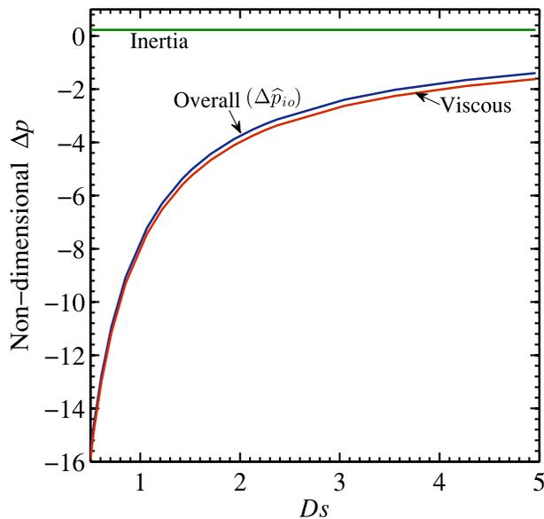
FIG. 9. Contribution of various forces within two static discs to produce the overall radial pressure difference  $\Delta\hat{p}_{io}$  over a range of dynamic similarity number  $Ds$ : prediction of the present CFD simulations for radial outflow. ( $\hat{r}_i = 0.528, \hat{b} = 0.008$ , and uniform velocity distribution at inlet:  $U_{r,i} = \bar{U}_{r,i}$ . Pressure differences are non-dimensionalized by  $\rho\bar{U}_{r,i}^2$ . Each curve contains data from 50 separate CFD simulations.)
