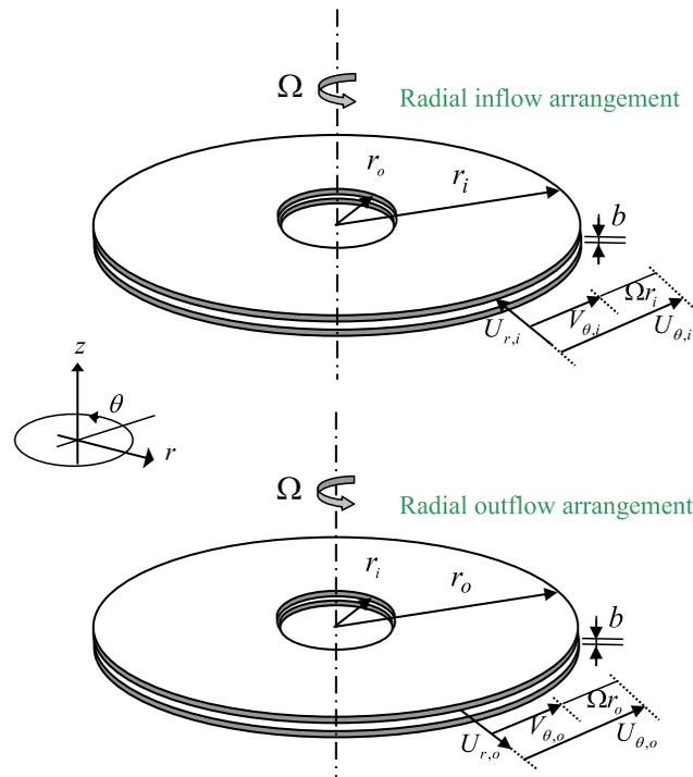
FIG. 1. Schematic diagram for the present physical configuration (the gap within the two discs, in relation to the radius, is exaggerated in the sketch for clarity) and two different flow arrangements (radial inflow and radial outflow).
