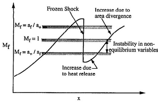
FIG. 13. Schematic structure of a supercritical condensation shock wave.
