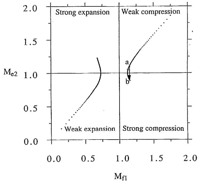
FIG. 8. Equilibrium Mach number downstream of condensation shocks in air-water mixture as a function of upstream frozen Mach number ( $p_1=2.5$  bar,  $g=0.99$ ,  $\Delta T_1=30$  K). Symbol: +:  $M_{f2}=1$ .
