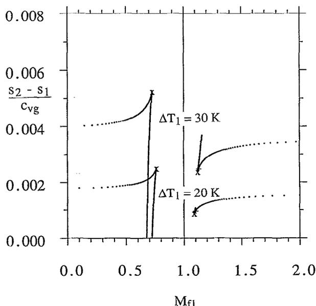
FIG. 10. Entropy rise across condensation shocks in air-water mixture as a function of upstream frozen Mach number ( $p_1=2.5$  bar,  $g=0.99$ ). Symbols: +:  $M_{f2}=1$ ,  $\times$ :  $M_{f2}=1$ .
