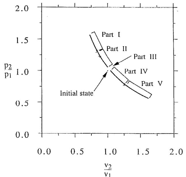
FIG. 9. Calculated downstream states of condensation shocks in air-water mixture with  $p_1=2.5$  bar,  $g=0.99$ ,  $\Delta T_1=30$  K. Symbols: +:  $M_{f2}=1$ ,  $\times$ :  $M_{e2}=1$ .
