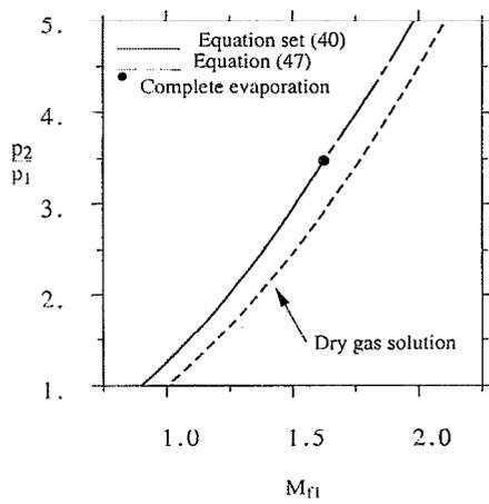
FIG. 5. Exact solutions for pressure ratios across aerodynamic shock waves in air–water mixture as a function of upstream frozen Mach number ( $p_1=1$  bar,  $T=293$  K,  $g=0.95$ ).
