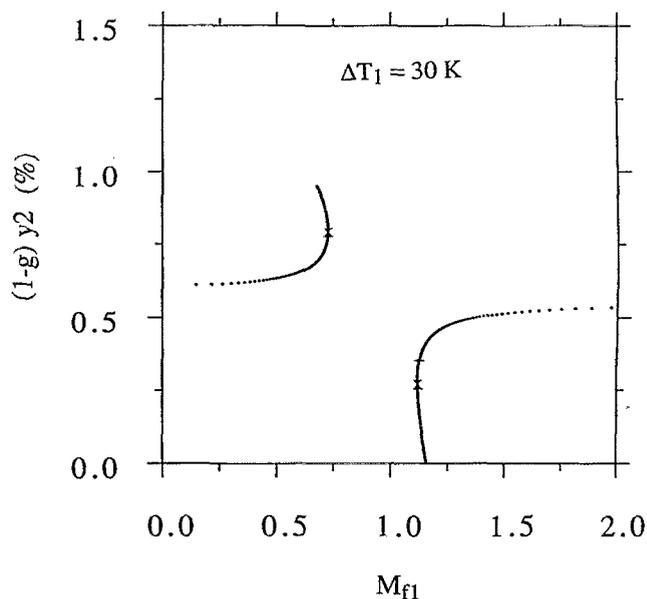
FIG. 11. Mass fraction of liquid phase condensed across condensation shocks in air-water mixture as a function of upstream frozen Mach number ( $p_1=2.5$  bar,  $g=0.99$ ). Symbols: +:  $M_{f2}=1$ ,  $\times$ :  $M_{f2}=1$ .
