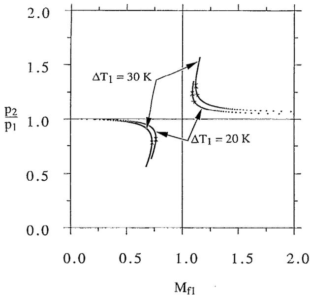
FIG. 7. Pressure ratio across condensation shocks in air-water mixture as a function of upstream frozen Mach number ( $p_1=2.5$  bar,  $g=0.99$ ). Symbols: +:  $M_{f2}=1$ ,  $\times$ :  $M_{e2}=1$ .
