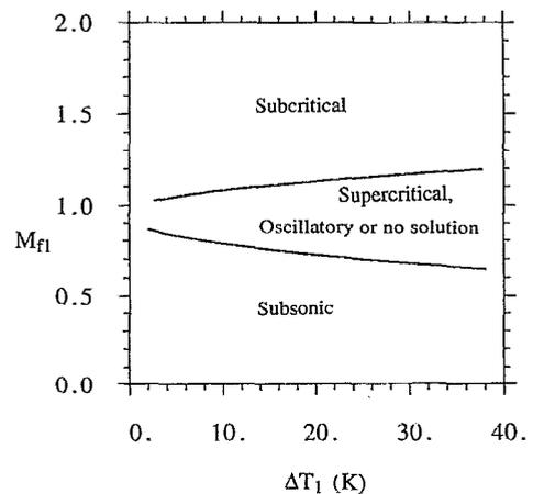
FIG. 14. Flow map for different condensation regimes in low-pressure, pure steam in terms of the frozen Mach number and subcooling at the Wilson point (results from the control volume analysis of Sec. V A).
