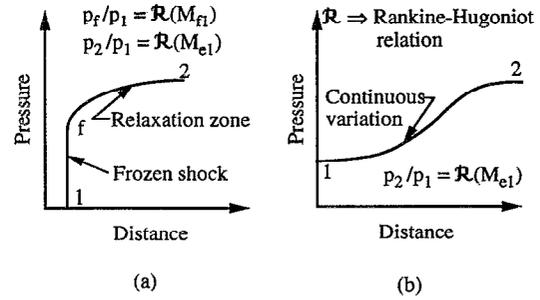
FIG. 3. Schematic structure of aerodynamic shock waves in a relaxing medium: (a) partly dispersed wave,  $M_{e1} > 1$ ,  $M_{f1} > 1$ , (b) fully dispersed wave,  $M_{e1} > 1$ ,  $M_{f1} < 1$ .
