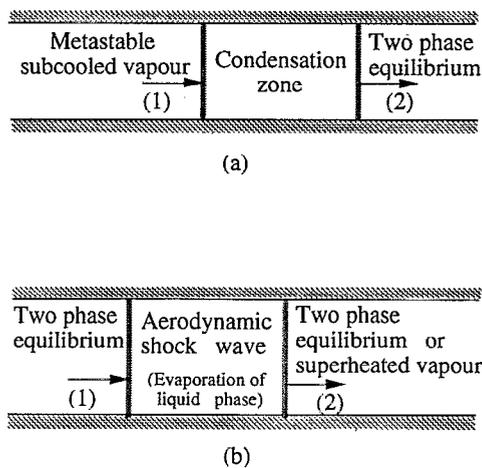
FIG. 1. Control volume analysis of discontinuities: (a) condensation shock, (b) aerodynamic shock wave.
