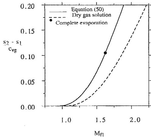
FIG. 6. Entropy rise across aerodynamic shock waves in air–water mixture as a function of upstream frozen Mach number ( $p_1=1$  bar,  $T=293$  K,  $g=0.95$ ).
