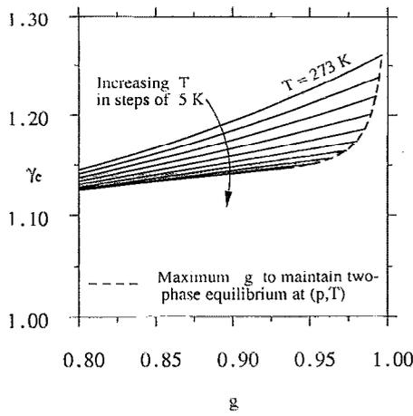
FIG. 2. Isentropic exponent in an equilibrium air-water mixture as a function of gas mass fraction ( $p=1$  bar, varying  $T$ ).
