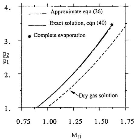
FIG. 4. Comparison of an approximate Rankine-Hugoniot solution with an exact jump condition for aerodynamic shock waves (air-water mixture,  $p_1=1$  bar,  $T=293$  K,  $g=0.95$ ).
