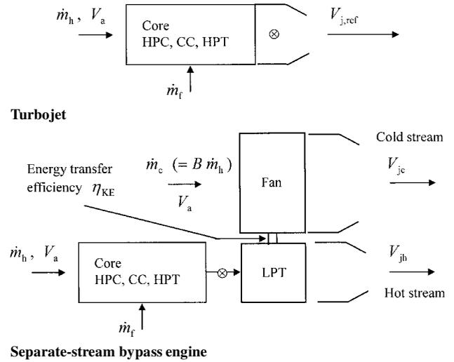
**Fig. 1 Schematic description of a separate-stream turbofan engine and an equivalent turbojet engine used for analysis; energy is the same at point ⊗ in both engines.**
