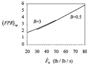
at the design point, the computed FPR then gives the optimum value independent of a specific mission of the aircraft.
