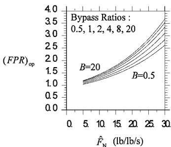
**Fig. 2 Variation of  $FPR_{op}$  with specific thrust in separate-stream bypass engines: prediction of Eq. (11);  $M = 0.82$ ,  $T_a = 216.65$  K,  $\eta_{KE} = 0.81$ , and  $\gamma = 1.4$ .**
