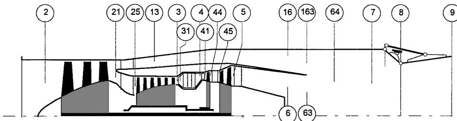
Fig. 6 Standard nomenclature for various locations in a mixed-stream turbofan engine (only half of the engine is shown).
