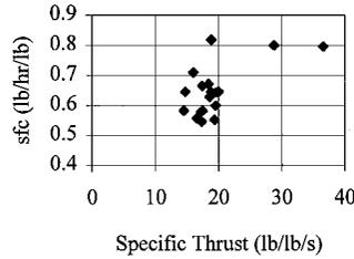
**Fig. 4 Data for various current civil turbofan engines under cruise conditions (typically 35,000 ft,  $M = 0.8-0.85$ ).**
