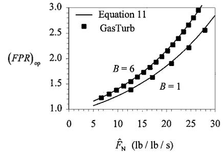
**Fig. 3 Comparison of present theory with numerical optimization results for  $FPR_{op}$  in separate-stream bypass engines. (Altitude = 11 km,  $M = 0.82$ , isentropic efficiency of compressors and turbines = 0.9).**
