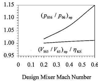
**Fig. 8** Effects of design mixer Mach number on the two characteristic ratios when  $FPR_{op}$  is achieved; for all calculations,  $M = 0.82$ ,  $B = 0.5$ ,  $\hat{F}_N = 60$  lb/lb/s, and component isentropic efficiencies = 0.9.
