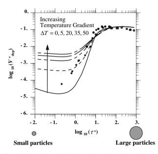
**Fig. 4** Effects of thermal diffusion on the predicted deposition rate.  $\Delta T = 0$  (*straight line*),  $\Delta T = 5$  K (*dashes*),  $\Delta T = 20$  K (*double dash straight line*),  $\Delta T = 35$  K (*broken straight line*),  $\Delta T = 50$  K (*single dash straight line*). For all computed curves,  $k_s^+ = 0$ ,  $\xi = 0$ , no lift force. Experiments [32] (*filled circle*)
