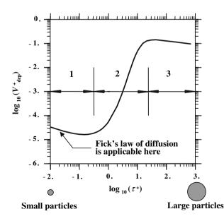
**Fig. 1** A typical variation in measured deposition rate with particle relaxation time. Regime 1: Turbulent diffusion, Regime 2: Turbulent diffusion—eddy impaction, Regime 3: Particle inertia moderated
