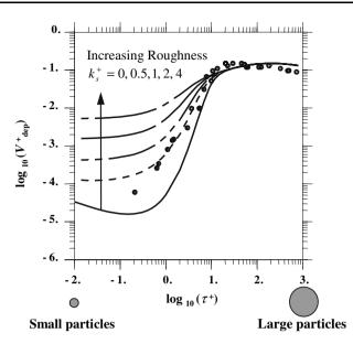
**Fig. 3** Effects of surface roughness on the predicted deposition rate.  $k_s^* = 0$  (straight line),  $k_s^* = 0.5$  (dashes),  $k_s^* = 1$  (double dash straight line),  $k_s^* = 2$  (broken straight line),  $k_s^* = 4$  (single dash straight line). For all computed curves,  $\Delta T = 0$ ,  $\xi = 0$ , no lift force. Experiments [32] (filled circle)
