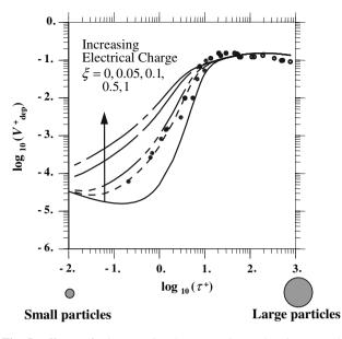
**Fig. 5** Effects of electrostatic charges (mirror charging) on the predicted deposition rate.  $\xi = 0$  (*straight line*),  $\xi = 0.05$  (*dashes*),  $\xi = 0.1$  (*double dash straight line*),  $\xi = 0.5$  (*broken straight line*),  $\xi = 1$  (*single dash straight line*). For all computed curves,  $k_s^+ = 0$ ,  $\Delta T = 0$ , no lift force. Experiments [32] (*filled circle*)
