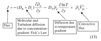
The coefficient of temperature-gradient-dependent diffusion,  $D_{\rm T}$ , in Eq. (13) is given by
