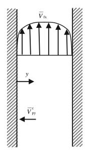
Fig. 7 Schematic for fully developed vertical upward flow
